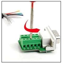
**Step 3:** Connect the PCB's female DB9 socket to the male DB9 connector on the USB-to-DB9 cable:
