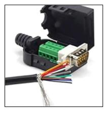
**Step 2:** Remove the PCB and connect the reader wires to the terminals according to the table:
