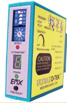
The ULTRAMETER™ display makes installation, set-up and troubleshooting easy. Each time a vehicle is moved onto the loop, the display indicates the sensitivity necessary to detect a vehicle. Simply set the sensitivity to the value displayed. Interference or crosstalk from adjacent loops or other sources are displayed as a constantly varying number on the ULTRAMETER™. This condition may be avoided by maintaining a minimum of 5 kHz separation in multi-loop applications.
