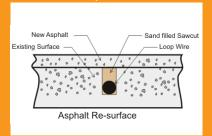
Saw cut existing surface 3/4" deep and place loop into bottom of saw cut. Place sand over loop wire to surface and pack tightly. Lay new asphalt.
