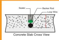
Cut 1" deep cut in existing surface, place 45° cut at the corners to relieve stress on the wire. Notch out for the "T" and place into the saw cut. Place backer material into saw cut over loop wire and push down tightly. Place a good grade sealer over the saw cut to
