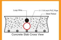
Ty-Wrap 1-1/4' PVC pipe to the top of the rebar in the size and configuration of your loop size. (example 4'x8') Then Ty-wrap the loop to the top of the PVC frame. This stabilizes the loop during the pour and separates it from the rebar
