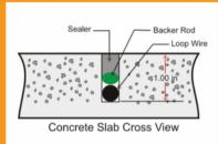
Cut 1" deep cut in existing surface, place 45° cut at the corners to relieve stress on the wire. Notch out for the "T" and place into the saw cut. Place backer material into saw cut over loop wire and push down tightly. Place a good grade sealer over the saw cut to seal surface.
