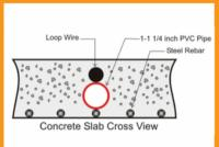
Ty-Wrap 1-1/4' PVC pipe to the top of the rebar in the size and configuration of your loop size. (example 4'x8') Then Ty-wrap the loop to the top of the PVC frame. This stabilizes the loop during the pour and separates it from the rebar.
