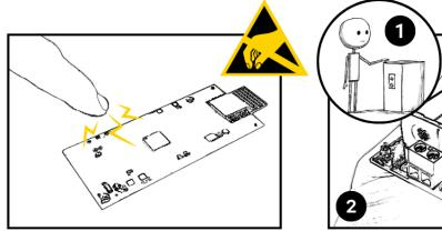
DON'T SHOCK ME! WEL-200T components are sensitive to static shocks (ESD)
