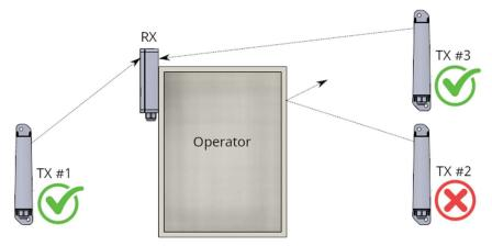
In the diagram, TX #1 and TX #3 have LINE OF SIGHT to the RX. TX #2 **does not** have LINE OF SIGHT to the RX because the operator will block the wireless signal. TX #2 may suffer from a poor connection and poor battery life.
