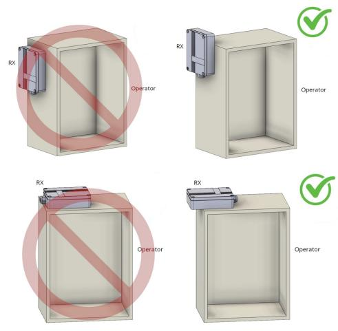
Even though there are 4 mounting holes on the RX, it's OK to just use 2 holes so that the RX will overhang the operator box as shown above. When mounting the RX, make sure the cable grip is facing down or to the side, never up - this will prevent water from getting in.
