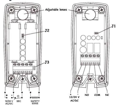
When transmitter frequency is set to low battery life will be increased. The range will be reduced at this setting. However when the transmitter is powered by 12/24 VDC or 24 VAC the range will be maximum regardless of the jumper setting.
